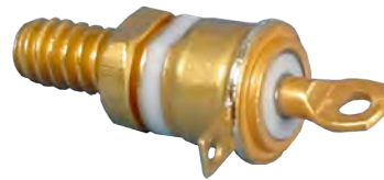
The example to the left is a 3BT-6 configuration, close on rise, gold contacts, close on rise at 82^{\circ}\text{C} \pm 4.4^{\circ}\text{C} , open at 65^{\circ}\text{C} \pm 4.4^{\circ}\text{C} .
