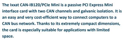
Galvanic isolation reliably enhances the protection of the device against damage to electronics caused by voltage peaks.
