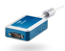
The Ixxat simplyCAN is an simple, uncomplicated and very costefficient way to connect a computer plug-and-play to a CAN bus network. It can be easily integrated into customer applications using a straightforward API and requires no driver installation for operation.
