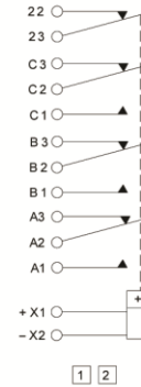
TERMINAL TYPE 5 3 PDT WITH SPST - N.C. AUX.
