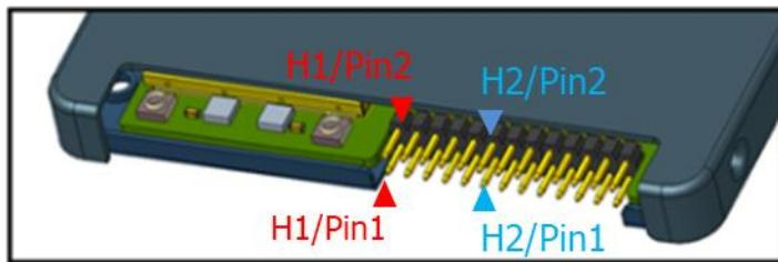
Pin Header 1 Recovery, Reset and External Reserved GPIO
