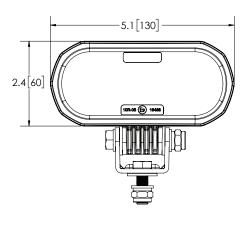
Measurements in inches (millimetres)
