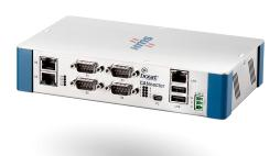
The Ixxat CANnector S is a versatile communication platform with many different interfaces. It seamlessly integrates several bus systems into a single device – ideal for logging and gateway applications.
